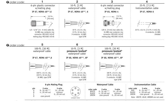
\*-Test pressure: 100 feet [30 meters] H2O (40 PSID) Test Medium: Air; Duration: 2 hours. \*\* -applies to stainless steel enclosure only. \*\*\*14-32 VDC for hazardous area option.
