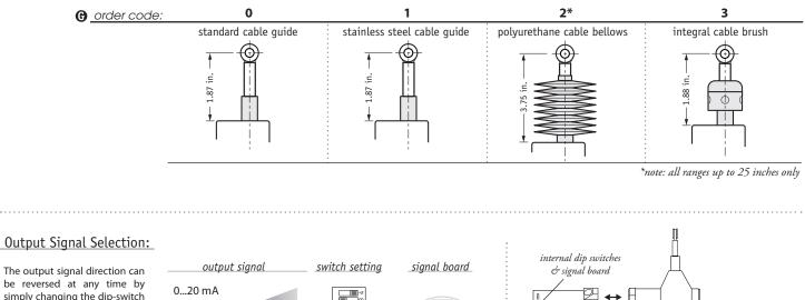
be reversed at any time by simply changing the dip-switch settings found on the internal signal board. After the settings have been changed, adjustment of the Zero and Span trimpots will be required to precisely match signal values to the beginning and end points of the stroke.
