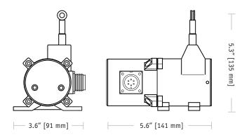
The PT8420 with its 4-20 mA feedback signal, is ideal for monitoring the stroke of a hydraulic cylinder and other applications requiring position data acquistion in harsh environments.
