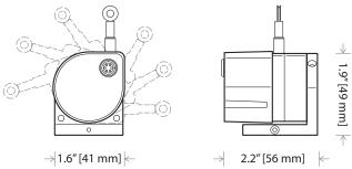
The MT2A is a member of our family of rugged, accurate miniature cable-extension position transducers designed specifically for test applications. One of the major benefits to this sensor its 2-axis 360° rotating mounting bracket to allow for fast and simple installation in any direction.
